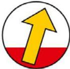
This feature also provides the line orientation arrow, which indicates direction of the utility. When signal distortion is detected the **circle fills up with red color** indicating that this particular area of the utility locate should be given proper attention to guarantee accuracy. Typically other adjacent utilities can cause distortion.
