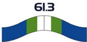
**The vLoc-5000 features Peak Indication.** Locating accuracy is guaranteed with the bar graph and numerical peak signal strength indication. The unique multi-color indication makes locating the exact peak a quick and easy task.
