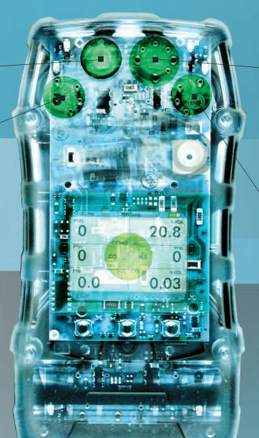
MSA XCell SO<sub>2</sub>, Cl<sub>2</sub>, or NH<sub>3</sub> Sensor
