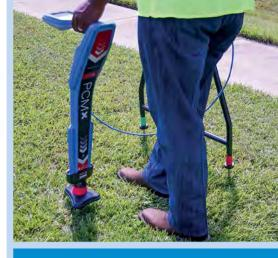
One second mapping measurements combined with simultaneous ACCA and ACVG data gathering makes surveying faster.
